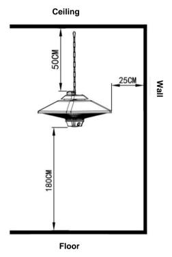
2. Now attach the supplied fastening chain to the holder hook by hooking one end of the chain into the holder hook with a carabiner.
